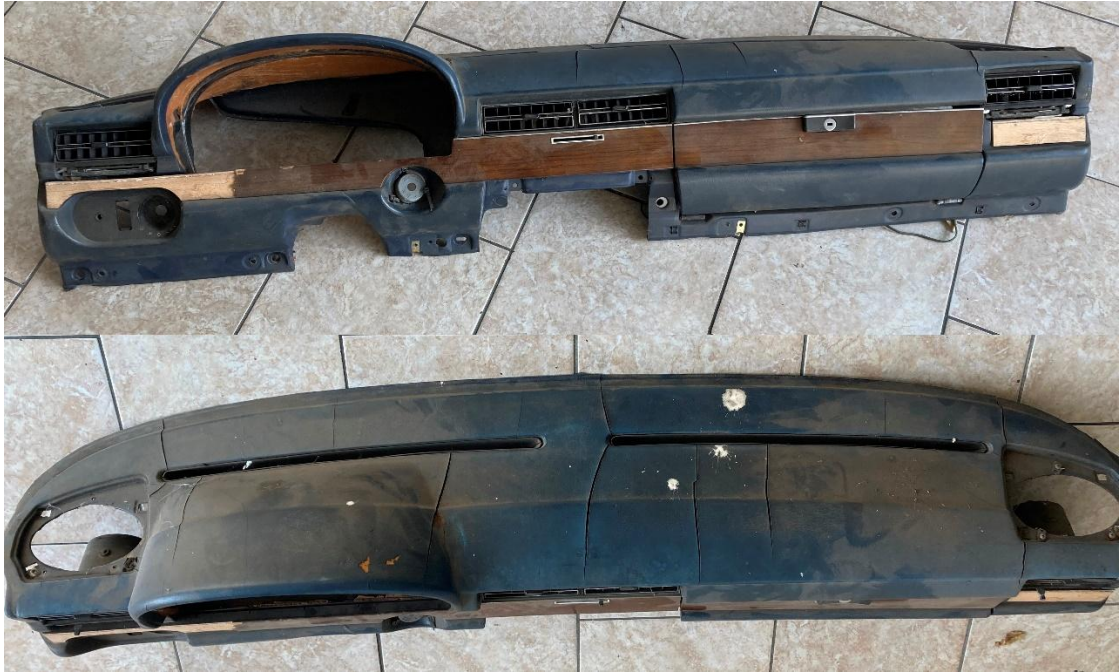
Figure 2. Dashboard removed for renovation
