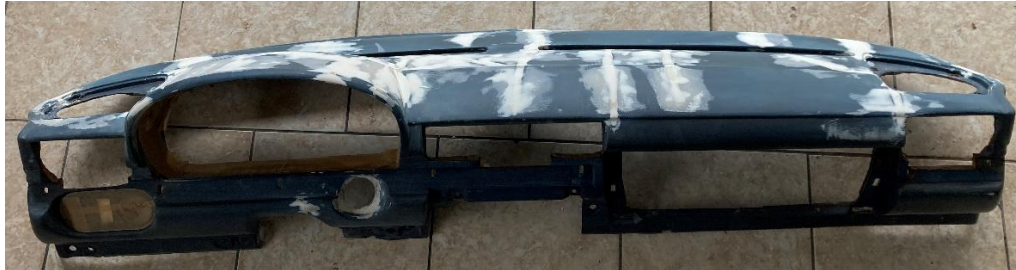
Figure 5. Primed surface prepared for texturing
