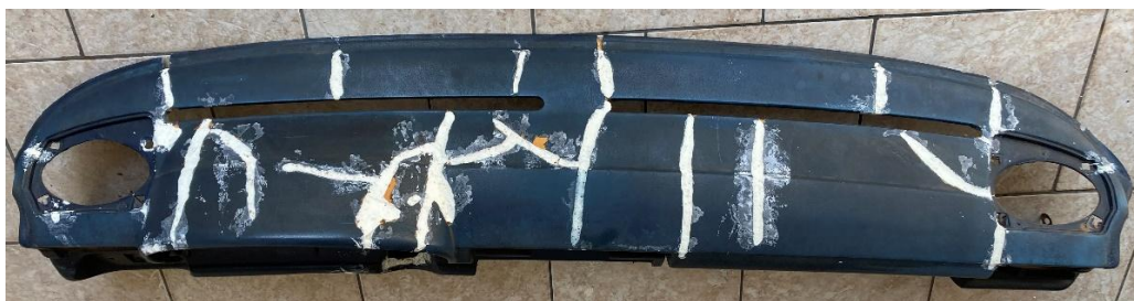
Figure 4. Polyurethane foam filled channels
