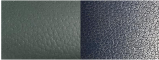
Figure 7. Original surface texture (right) and surface sprayed with textured polyester filler (left)
