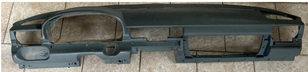
Figure 6. Textured polyester-sprayed surface
