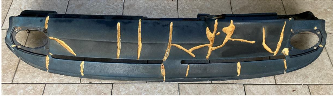
Figure 3. U-shaped cracks milled into the dashboard
