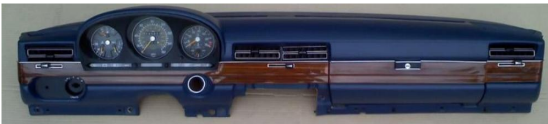
Figure 8. Assembled complete restored and painted dashboard
