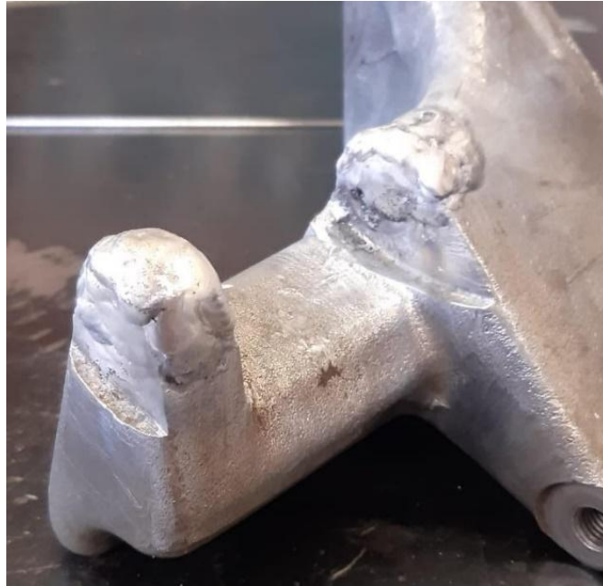
Figure 4. Surface elements filled with TIG welding
