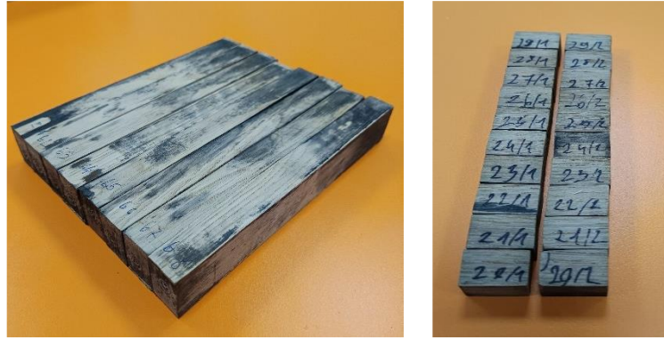
Figure 2. Images of some specimens after pleating (left) and after cutting for compression test (right)
