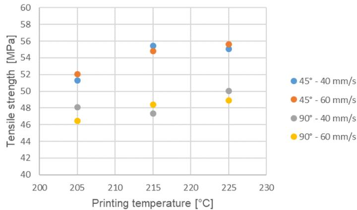
Figure 4. Tensile strength as a function of printing settings
