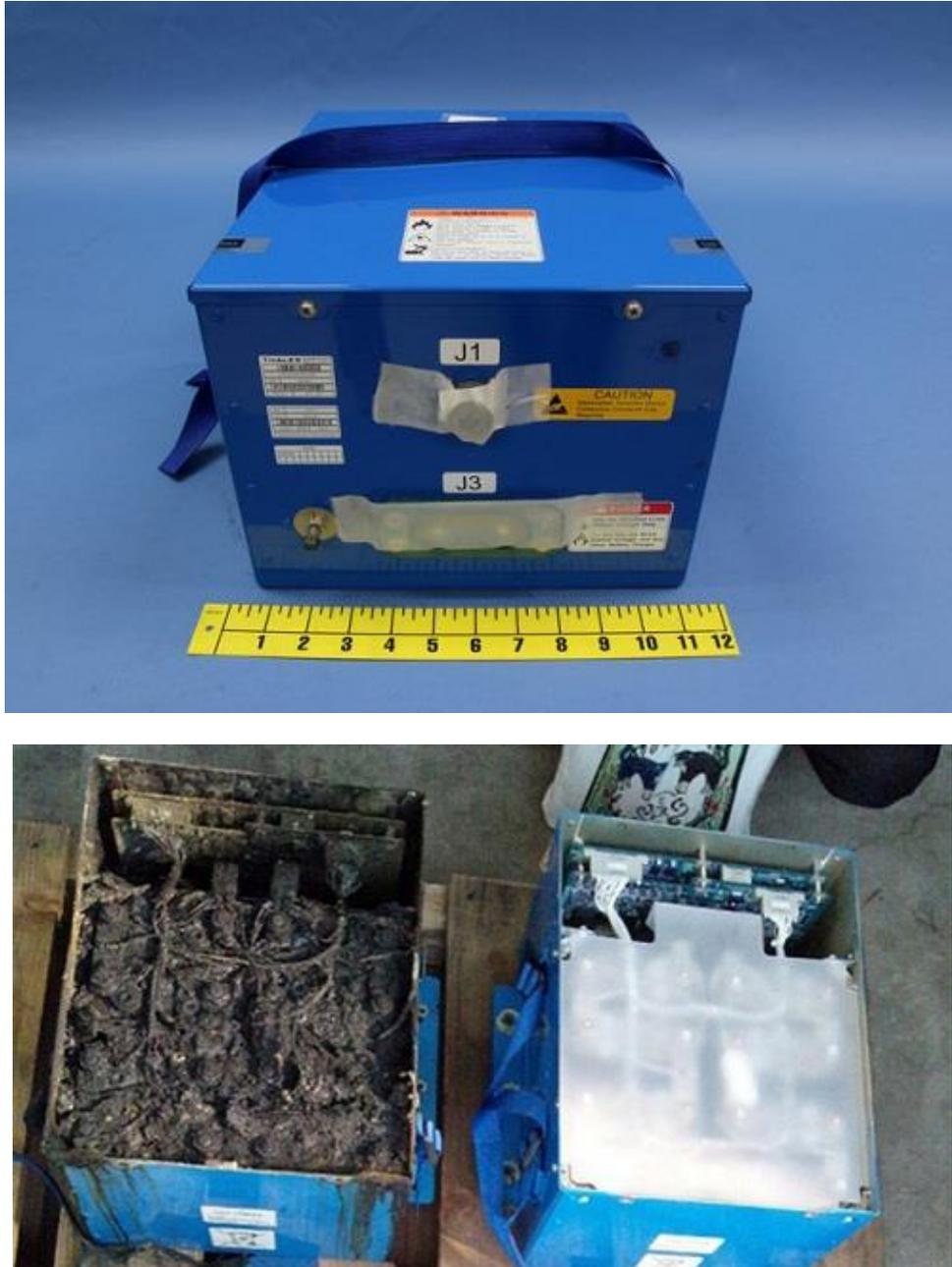
Figure 1. Fire of the Li-ion battery [3]
