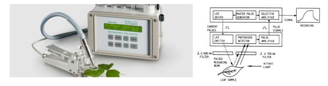
Figure 4: MINI-PAM Photosynthesis yield analyzer and the schematic view of the PAM measuring principle (source: http://www.odb.com.tw/)
