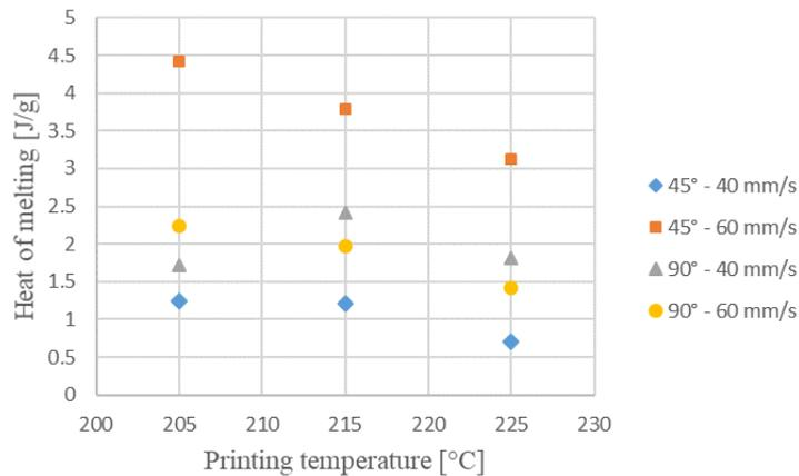
Figure 7. Heat of melting as a function of printing settings
