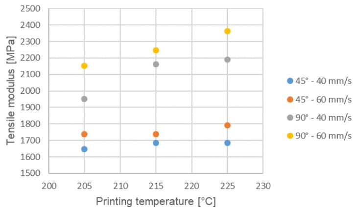
Figure 3. Tensile modulus as a function of printing settings
