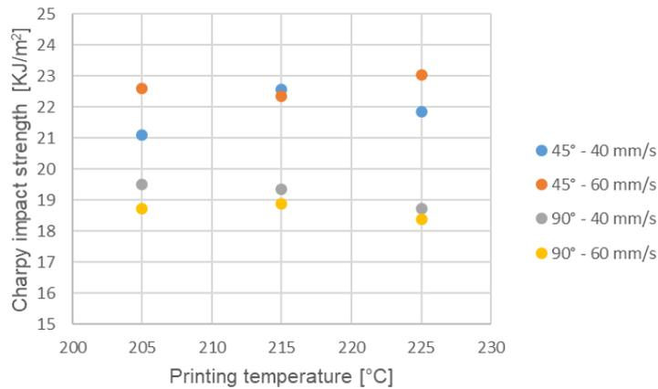
Figure 2. Impact strength as a function of printing settings
