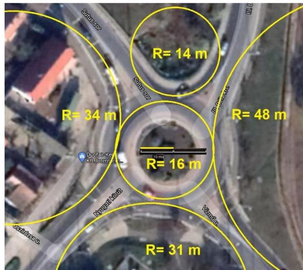
Figure 2. The satellite photograph (by Google) of the roundabout used for the test. The inscribed circles of the most often used paths are drawn by yellow lines.
