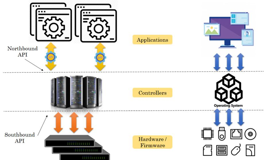
Figure 2. SDN Stack VS operating systems abstraction layers
