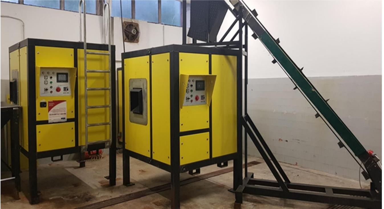
Figure 1. "ROPAL 1000" abrasive peeling machine
