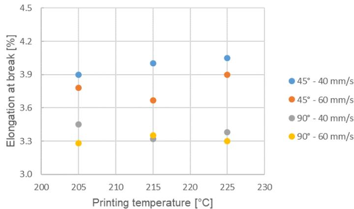
Figure 5. Elongation at break as a function of printing settings
